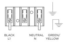
**NOTE:** This electrical service consist of 2 current carrying conductors (L1 and Neutral) and a separate conductor for earth ground.
