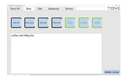
The name of the recipe tells you the strength of the coffee, the amount of water and the applied filter type.
